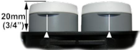
Install two GEOSATpro Mini Bullet LNBFs into the Twin LNBF Clamp, align the centering line on the top of each LNBF with the centering pointer on the clamp. Slide the LNBF forward towards the reflector so the white front face of the LNBF cap is slid 20mm (3/4") forward of the clamp towards the reflector. Securely tighten both clamp screws (2).
