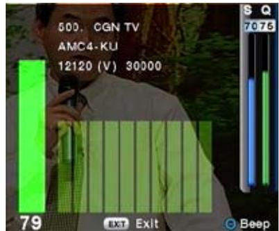
***The Signal Level (S) is not important in detecting the satellite. Signal Level readings indicate a connection to a functioning LNB, not the detection of the correct satellite.***
