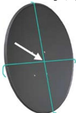
If the reflector is warped, pick up the dish by the edges like a steering wheel and quickly thrust the reflector away from your body while holding the edges of the dish like passing a basketball. This action will cause the reflector to flex and it will spring back into the factory pressed shape. Lay the reflector face down and observe if the edges are now laying perfectly flat. If not, repeat the flexing process until the reflector edges are uniformly flat.
