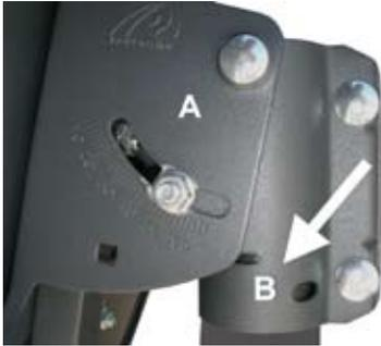
Most installations in the US and Canada will use Elevation Scale "A" type assembly. The dish has been correctly assembled for Measuring the Dish Elevation Angle using Scale A (10 - 60 degrees) if an upside letter B is visible stamped on the Post Clamp on the left side of the Post Clamp.
